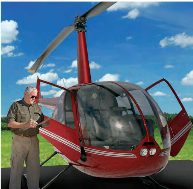
Figure 8-1. The pilot in command is responsible for the airworthy condition of the aircraft and using checklists to ensure proper inspection of the helicopter prior to flight.
