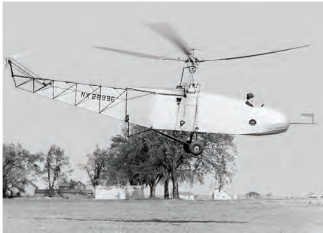
Figure 1-8. Igor Sikorsky designed the VS-300 helicopter incorporating the tail rotor into the design.
